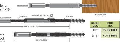
For sleeved posts with an outside diameter of greater than 4-1/2", use the Push-Lock<sup>®</sup> Turnbuckle with Extended Length Hanger Bolt. The extended length hanger bolt is designed to reach past sleeves and drywall to find the wood post or frame underneath.
