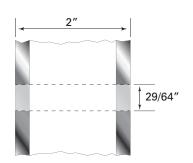
Drill and tap 5/16-24 threaded hole on the inside of the other end post for the Push-Lock® fitting.
