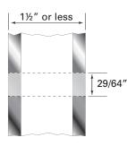
Drill and tap 5/16-24 threaded hole on the inside of the other end post for the Push-Lock<sup>®</sup> fitting.
