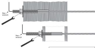
2. Tension all cables to desired amount in sequence, beginning with the center cables, moving up and down toward the top and bottom. As you tension each cable, give it a sharp pull downward mid-span to help set the wedges, then re-tension as necessary in the same sequence.
